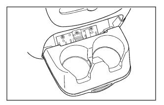
Pull down the door on the back of the center console to use the rear seat cupholders.
